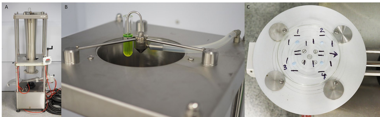
Fig. 1 The Potter Tower. The Potter Tower is shown (A) with a close up on the nozzle and three arms with the adjustment screws on the three stands (B), and the coverslip positioning on the spray table (numbered 1–4), raised on Bostik Blu Tack ® , with four moveable discs to secure the Petri dish (C)
