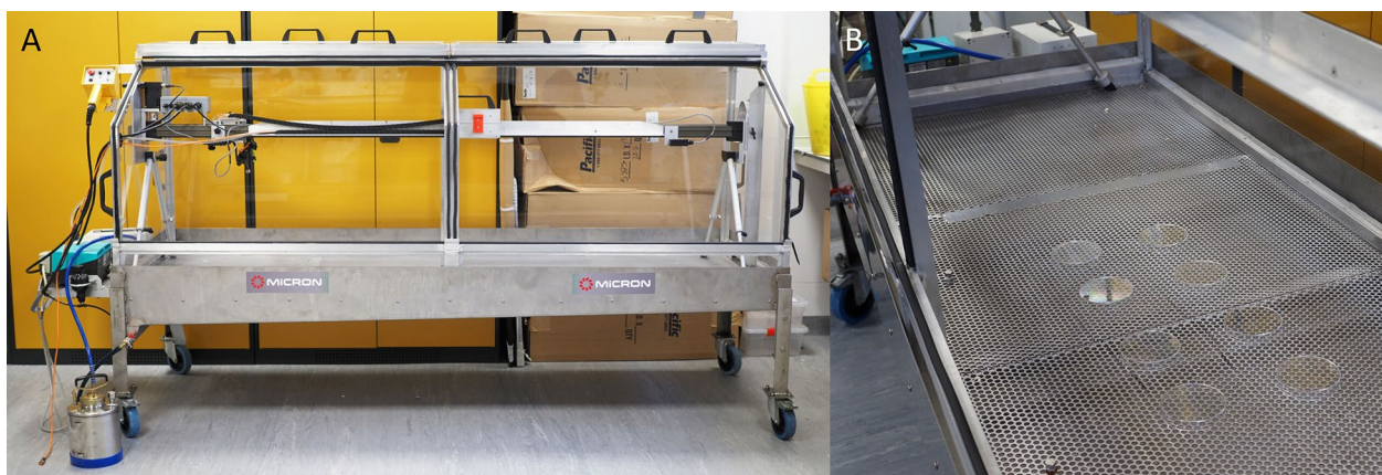
Fig. 2 The Horizontal Track Sprayer developed by Micron Sprayers. The Track Sprayer is shown empty (A) and with eight samplers arranged on the track for calibration (B)
