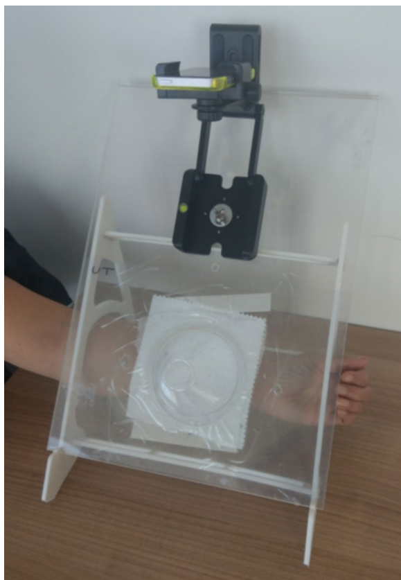
Fig. 1 Experimental rig for video cone test analysis. The test netting is sandwiched between two pieces of 3-mm acrylic mounted at 45° and containing a 9-cm hole to allow exposure to the host stimulus scent. The host rests its arm below the scent stimulus hole, and mosquitoes are not able to contact the host arm. A smartphone is placed above the cone and immobilised at a fixed distance and angle using a z-clamp
